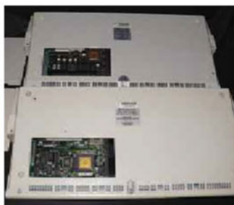
◀ The trapdoor slot under the machine. Note the connector on the Phase 5 card in the upper machine, which allows the connection of a daughter card that is secured in the exposed bay when the rear panel blanking plate is removed
