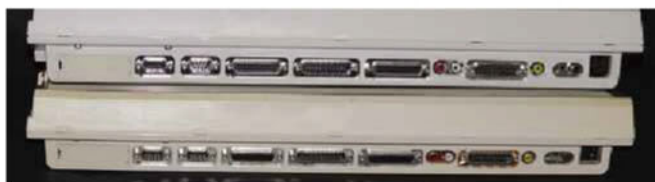
▲ From left to right – Expansion blanking plate, Mouse/joystick port 1 and 2, external disk drive connector, serial port, parallel port, audio out R&L, RGB video out, composite video out, RF out and power in.
