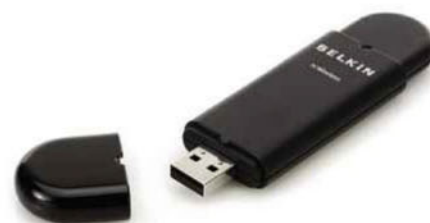
▲ If you don't have a wired network, but still want to use this technology you could use a Belkin F5D8053 v3 USB wireless adapter to add WiFi to your DS115j. Synology supports many more wireless USB adapters, for a full list check their website ( www.synology.com/en-us/knowledgebase/faq/427 ).
